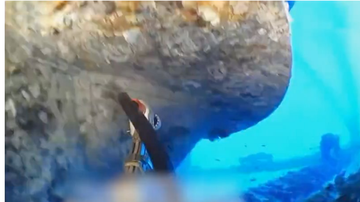
Eddy Current (EC) probe deployment using an ROV manipulator
