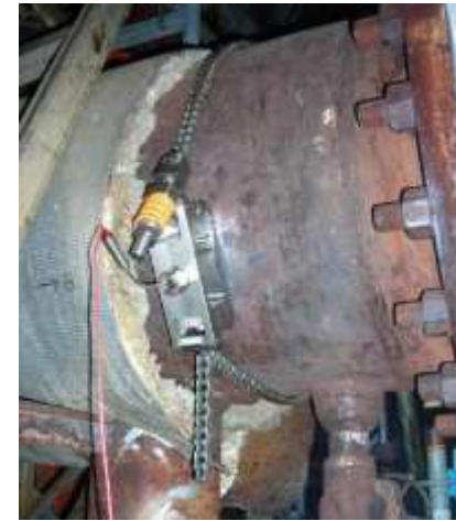
High-temperature UT probe (courtesy GE/iicor)
