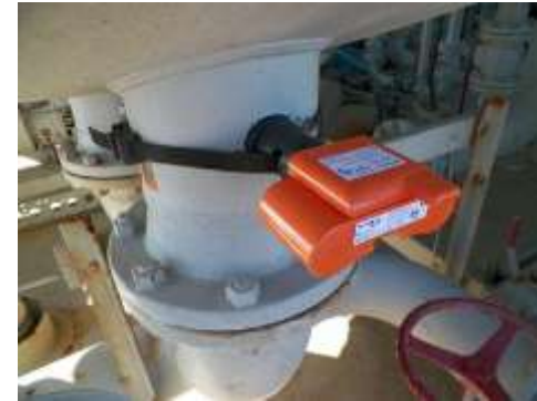
EMAT version, strapped on pipe, to avoid welding (courtesy Permasense)
