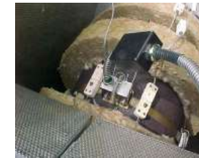
PEC Monitoring (courtesy Shell)
