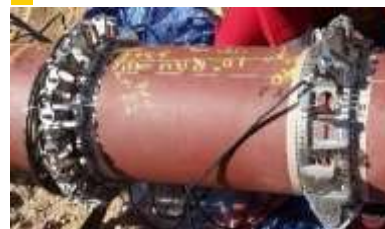
GWT (courtesy ClampOn/PDO)
