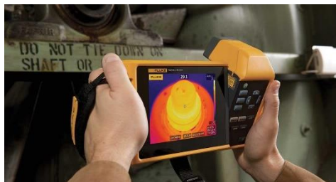
Infrared (IR) Thermographic Inspection
